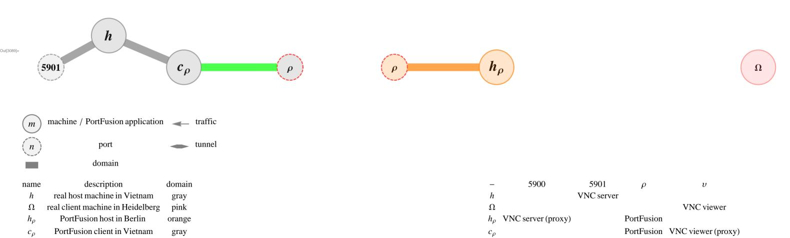
we connect PortFusion client  $c_{\rho}$  with PortFusion host  $h_{\rho}$  and open port  $h_{\rho}$ :5900 as a proxy of our VNC server on h at h:5901 >> this opens a tunnel through the firewall of real host h <<
